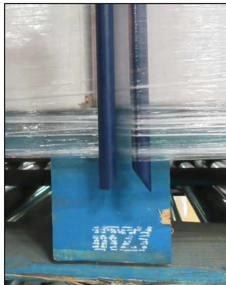
Figure 9 – Piercing Finger Position on the Film Cable.
